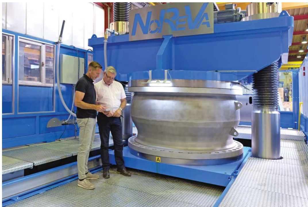
A Semi-Automatic Ventil VCB-3500 used in daily operation testing NOREVA Check Valves 20"- 80". Photo: Ventil Test Equipment
