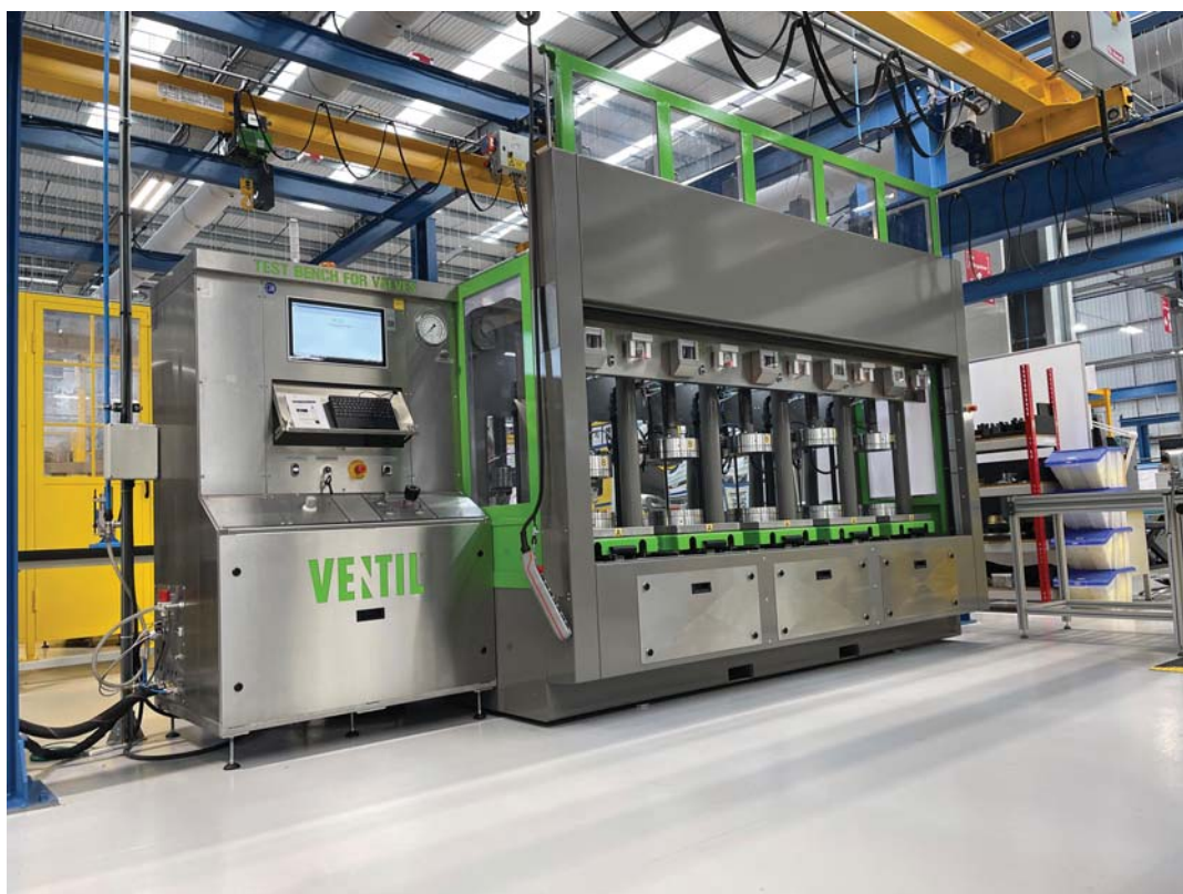
Customised solutions with 2 to 6 test stations for faster and repeatable performance. Photo: Ventil Test Equipment
